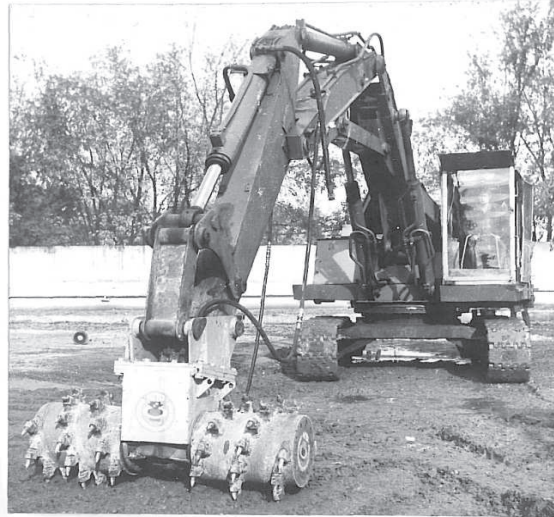
Figure 13 A prototype of a universal cutterhead with cutters installed on the base machine (single-bucket excavator)
