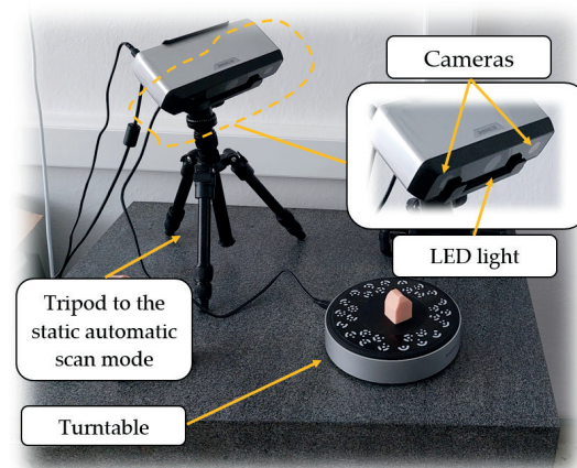
Figure 2 EinScan - SP 3D scanner
