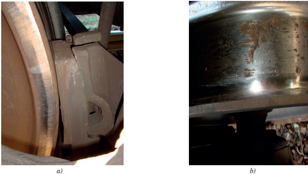
Figure 1 The elements of the brake pad/wheel tribotechnical assembly that are inoperable due to the BLT design features; a) without a clearance between the pad and a wheel when the brakes are released; b) high-temperature damage on the wheel surface
