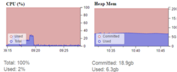
Figure 5. CPU and Elasticsearch utilization in test 2 (many sources)
