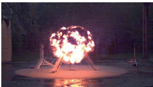
Figure 13 Test of the explosion regularity of Semtex 10-SE, t = 5.236 \text{ ms}
