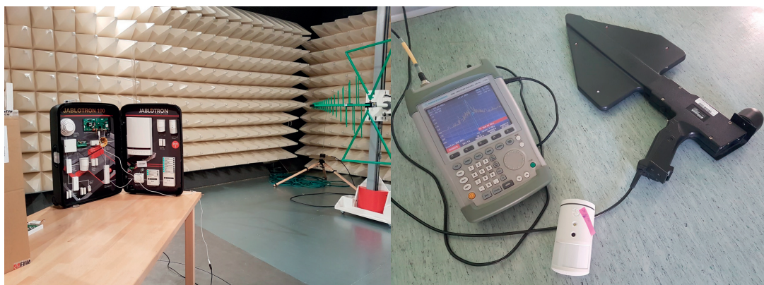
Figure 1 The Franconia non-reflecting chamber and the spectrum analyzer and the antenna during testing
