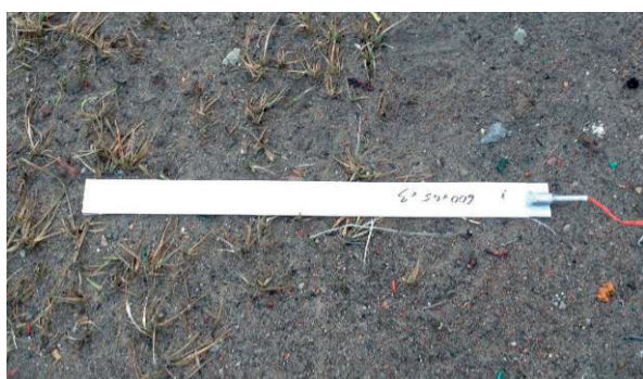
Figure 2 Detasheet explosive Semtex PI SE
