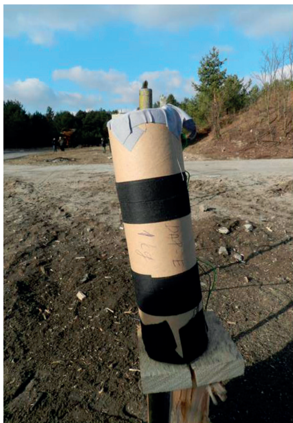
Figure 4 Explosive DAP - E weight 1000 g for field test
