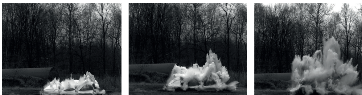
Figure 10 Time sequence of charge explosion - 3 water bag placed
