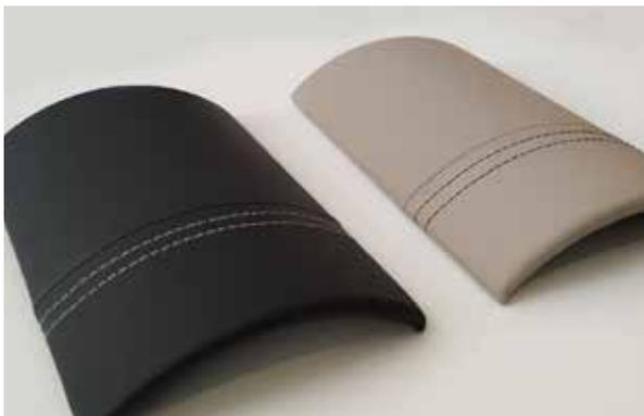
The Nanocleanleather project set out to develop leather with anti-soiling properties (dirt-repellence and easy cleaning) and self-cleaning (photocatalytic degradation of contaminants on the surface of the leather) for the automotive sector (specifically seat covers, steering wheels, dashboards and door panels) using nanostructured additives.
