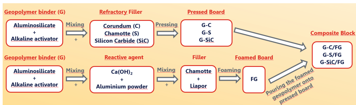
Figure 1. Scheme for preparation of a composite blocks
