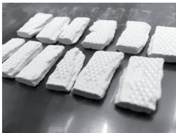
Figure 7. Comparison of the ribbons from Gerteis, Mini-Pactor [250/25] ([A], SCF 9.6 kN/cm) and Alexanderwerk, WP 200 [200/75] ([B], pHYD 160 bar).
