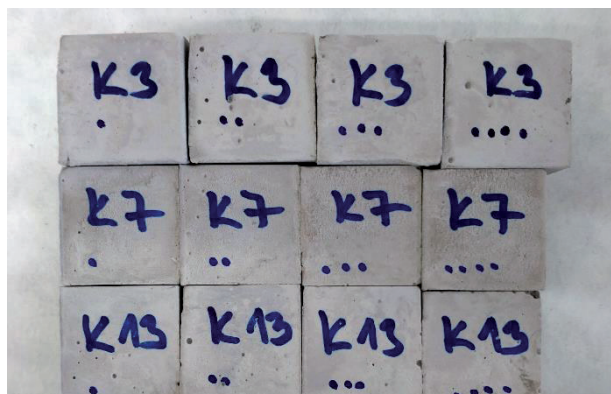
Figure 3. Visible expansion of sample K3 after 7 days
