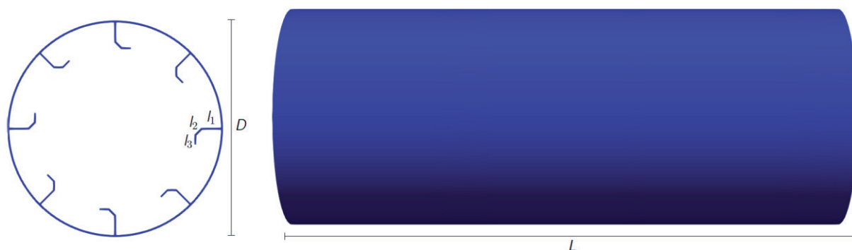
Figure 3. Geometry of the rotary kiln according to Silveira.
