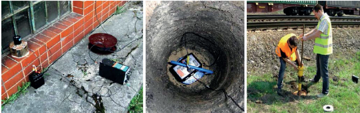
Fig. 3 Accelerometers installed in soil and on structure, ISM procedure
