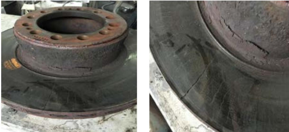
**Figure 1** Defects of the brake disk of a truck
