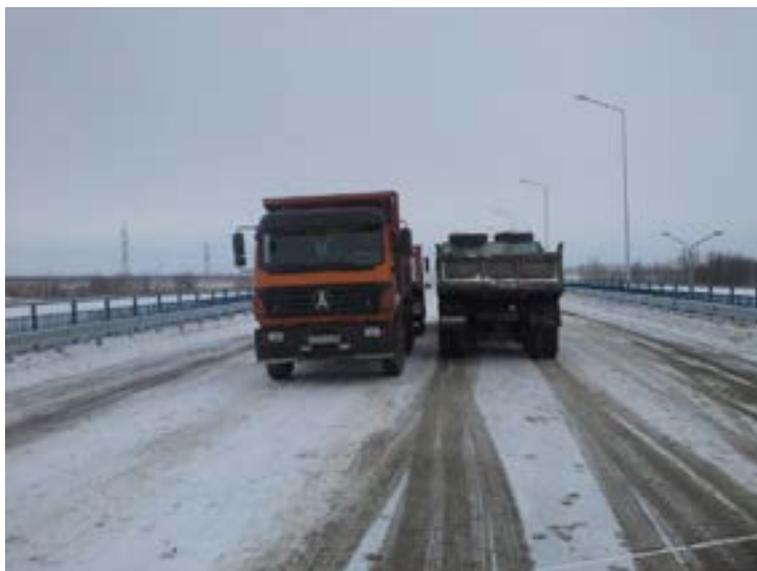
**Figure 6** Vehicles are located at the longitudinal axis of superstructure No. 1 at the third stage of testing
